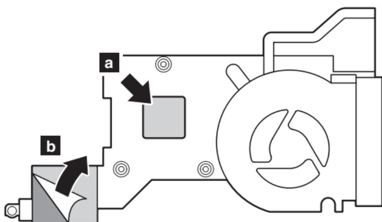
Figure 2. Fan assembly, long
